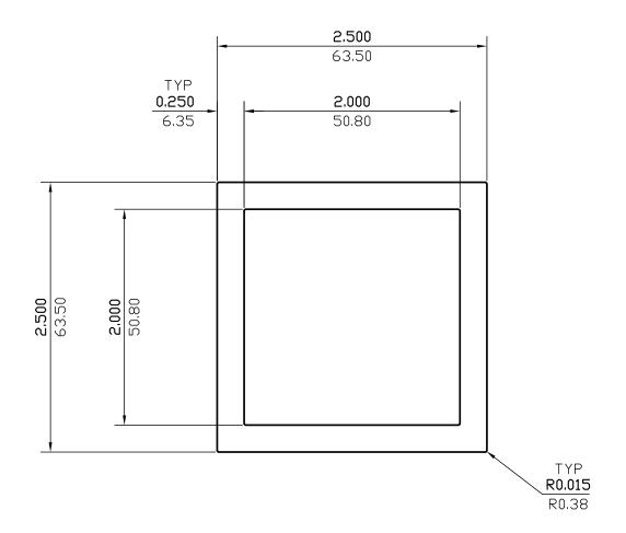
0.250 (6.35) WALL THICKNESS EXCEPT AS SHOWN DATE REV DESCRIPTION BY 1451.621 мм.<sup>2</sup> \_IN.<sup>2</sup> 2.250 EST.AREA EST.AREA 3.951 2.655 EST.WT. LBS/FT. EST.WT. KG/M. 17.948 455.892 EST.PER. EST.PER. MM. 9.974 253.3 OUT PER. OUT PER. MM. 3.523 89.487 C.C.D. C.C.D. 6061 **FINISH** M/F ALLOY SCALE 1:1 DWN BY P.M. DATE 11/02/2011 FACTOR CKD BY
