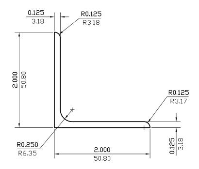
DATE REV DESCRIPTION BY 03/20/23 2 REMOVED ALLOY NDZAL 08/28/03 UPDATED DRAWING L.G. 316.829 мм.2 0.491 IN.<sup>2</sup> EST.AREA EST.AREA 0.877 0.589 EST.WT. LBS/FT. EST.WT. KG/M. 7.785 197.749 EST.PER. MM. EST.PER. OUT PER. MM. OUT PER. 2.828 C.C.D. 71.842 C.C.D.
