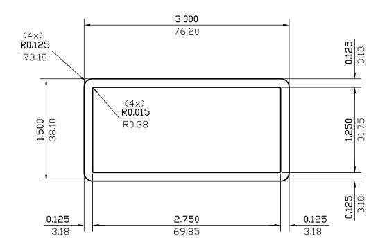
0.125(3.18) WALL THICKNESS EXCEPT AS SHOWN DATE REV DESCRIPTION BY 03/15/23 REMOVED ALLOY NDZAL мм.<sup>2</sup> 676.959 ın.<sup>2</sup> 1.049 EST.AREA EST.AREA 1.874 1.259 EST.WT. LBS/FT. EST.WT. KG/M. 16.760 425.695 EST.PER. MM. EST.PER. 8.785 223.1 OUT PER. MM. OUT PER. 3.270 C.C.D. 83.064 C.C.D. FACTOR 13 **FINISH** M/F ALLOY & TEMP. 1:1 DWN BY C.P.SCALE DATE 03/02/2004 CKD BY
