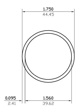
AS SHOWN WALL THICKNESS EXCEPT AS SHOWN DATE REV DESCRIPTION BY 318.671 мм.2 EST.AREA 0.494 EST.AREA 0.867 0.583 EST.WT. LBS/FT. EST.WT. KG/M. 10.399 EST.PER. 264.126 MM. IN. EST.PER. 5.498 139.6 OUT PER. IN. OUT PER MM. 1.750 44.450 C.C.D. C.C.D. FACTOR 18 FINISH PAINT ALLOY & TEMP. 6061 1:1 DWN BY  $\mathbf{C}.\mathbf{P}.$ DATE 08/30/2001 CKD BY SCALE
