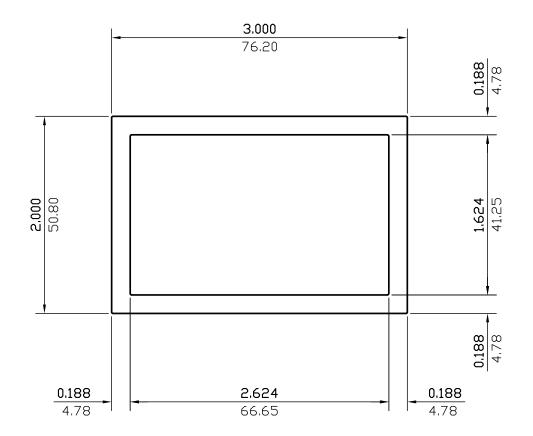
(AS SHOWN) WALL THICKNESS EXCEPT AS SHOWN DATE REV DESCRIPTION BY 03/14/23 REMOVED ALLOY NDZAL 1121.700 мм.2 <sub>\_IN.</sub>2 1.739 EST.AREA EST.AREA 3.105 2.086 EST.WT. LBS/FT. EST.WT. KG/M. 18.496 469.798 EST.PER. EST.PER. MM. 10.000 254.0 OUT PER. OUT PER. MM. 3.606 91.581 C.C.D. C.C.D. FACTOR 9 FINISH M/F ALLOY & TEMP.
