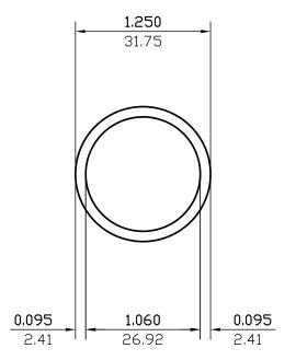
0.095(2.41)WALL THICKNESS EXCEPT AS SHOWN DATE REV DESCRIPTION BY 03/10/23 REMOVED ALLOY NDZAL 222.396 мм.2 \_IN.2 0.345 EST.AREA EST.AREA 0.6050.407 EST.WT. LBS/FT. EST.WT. KG/M. 7.257 184.330 EST.PER. MM. EST.PER. 3.927 99.746 OUT PER. MM. OUT PER. 1.250 31.750 C.C.D. C.C.D. FACTOR 18 **FINISH** M/F ALLOY & TEMP. 1:1 DWN BY C.P. SCALE 05/04/00 CKD BY DATE
