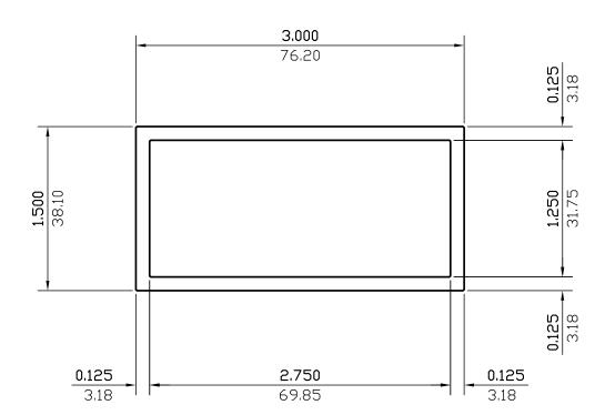
0.125(3.18) WALL THICKNESS EXCEPT AS SHOWN DATE REV DESCRIPTION BY 03/14/23 REMOVED ALLOY NDZAL 685 мм.2 1.063 IN.<sup>2</sup> EST.AREA EST.AREA 1.254 1.866 EST.WT. LBS/FT. EST.WT. KG/M. 17.000 431.8 EST.PER. MM. EST.PER. 9.000 228.6 OUT PER. MM. OUT PER. 3.354 C.C.D. 85 C.C.D. FACTOR 14 **FINISH** M/F ALLOY & TEMP. 1:1 DWN BY  ${f C.P.}$ SCALE DATE 11/30/99 CKD BY
