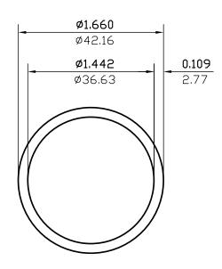
0.109(2.77)WALL THICKNESS EXCEPT AS SHOWN DATE REV DESCRIPTION BY 03/10/23 REMOVED ALLOY NDZAL 342.657 мм.2 ın.<sup>2</sup> 0.531 EST.AREA EST.AREA 0.627 0.933 EST.WT. LBS/FT. EST.WT. KG/M. 9.745 247.529 EST.PER. MM. EST.PER. 5.215 132.5 OUT PER. OUT PER. MM. 1.660 42.164 C.C.D. C.C.D. **FINISH** M/F ALLOY FACTOR 16 SCALE 1:1 DWN BY D.L.06/21/2017 CKD BY DATE
